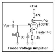
No load is shown for this amplifier, which would normally be the grid of the following tube, or actually the grid resistor, since the grid has a very high input resistance. The output impedance of the amplifier is the plate resistance in parallel with the plate resistor, about 5.9k, satisfactorily lower than the input resistance of the following grid. Resistance-capacitance coupling works much better for triodes than for transistors, and is usually very satisfactory.
