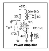
At low plate and screen voltages, a remarkable oscillation is observed. This was seen at about 70 V supply voltage, much less than would normally be used. The oscillation at about 250 Hz was
