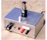
The voltage regulator requires a certain minimum current (about 5 mA) to function properly. If you are only drawing a few milliamperes from the supply, connect a 12k bleeder resistor across the output. Otherwise, the regulator will not adjust down to the lower voltages. Or,  $220\Omega$  and 10k fixed resistors, and a 15k pot, could be used at the voltage regulator, which would draw the necessary minimum current. The VR tube can be replaced by a high-voltage Zener diode.
