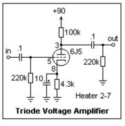
A different resistance-coupled triode voltage amplifier is shown in the diagram on the left. The resistance "seen" by the 0.1  $\mu$ F coupling capacitors is 100k || 220k or 68.8k. The corner frequency of this RC filter is  $1/2\pi$ RC = 23 Hz, sufficiently low for an audio amplifier. The corner frequency of the cathode bypass is 48 Hz. The predicted gain is roughly  $g_m = 3.0$  mS times 7.7k||100k||220k = 6.9k, or -21. It drops to about -6.9k/4.6k = -1.5 if the cathode is not bypassed.
