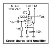
The modern space-charge grid tetrodes allow us to work with a tube type from the dim past of vacuum tubes. Most texts never mention this kind of tube.
