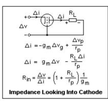
It is most enlightening to consider the circuit as a common-cathode amplifier driving a common-grid amplifier. To estimate the gain of the common-
