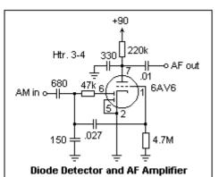
A detector-amplifier circuit is shown at the left. This circuit is fed by a signal generator at AM in, and the audio output is taken from AF out. The amplifier uses grid-leak bias, which effectively clamps the peak of
