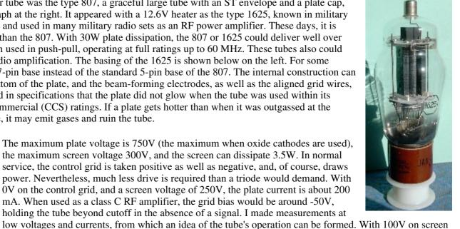
and plate, I found a transconductance of 2.8 mS and a plate resistance of 39k. As a triode, the amplification factor is 8, the plate resistance 2900Ω, and the transconductance about 3 mS (not all at the same point). The tetrode dip occurs only below 50 mA plate current, and was obvious in my measurements. Incidentally, I found a large copper-plated spring clamp to make the plate contact, lacking a proper plate cap.
