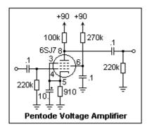
A pentode voltage amplifier using a 6SJ7 is shown at the left. The AC gain of this amplifier is close to  $g_m$  = 1.6 mS times 68.8k, or -110. It won't be quite this high with a 90V B+, but will still give a lot more gain than the triode amplifier. My 6SJ7 gave a gain of -60 at  $V_{bb}$  = 90 V, and  $V_p$  was 27.2 V, showing that the plate current, 0.63 mA, should be reduced a little to raise the plate to about 45 V. The 6SJ7 tested was very close to specifications, despite its age.
