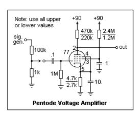
current to permit a large plate resistor for high gain, so the screen voltages are quite low. No load is shown for the amplifier, but it would usually be a high-impedance grid.
