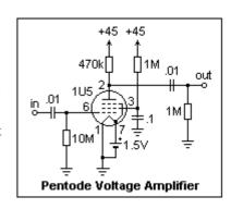
DMM or scope, since the bias conditions will be disturbed. However, you will find that the amplifier works very well. Measure the gain the usual way, with a function generator and oscilloscope.
