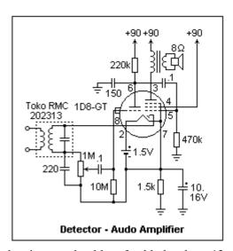
I used the P-T31 that has been used in other places, which matches  $8\Omega$  to  $5 \text{ k}\Omega$ . The load resistance should preferably be about 12 k $\Omega$ . However, it drove a good speaker at considerable volume with a rather small input. A three-tube battery radio could be made with this tube, an IF amplifer stage, and a pentagrid converter, a tube type which will be treated next.
